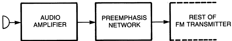
Figure 6-18 FM transmitter with preemphasis network.
